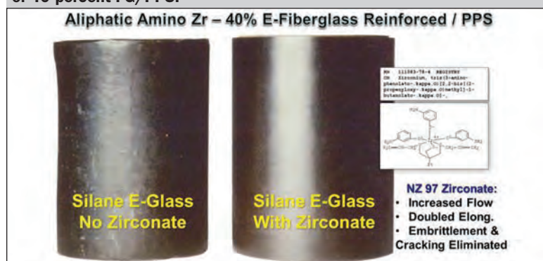
Fig. 20: An aromatic amino zirconate improves the flow and properties of 40-percent FG/PPS.
