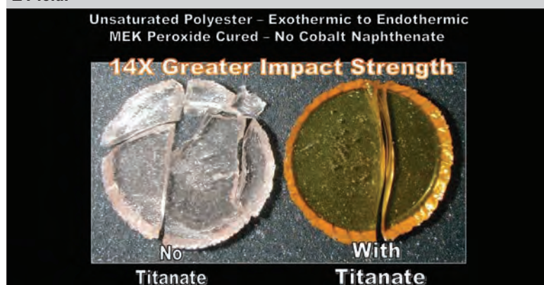
Fig. 16B: Titanate increases impact strength of unsaturated polyester 14-fold.
