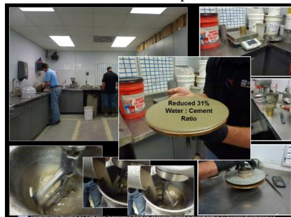
Fig. 11 – Titanate treated Portland cement (ASTM C150 Type I) reduces the cement H 2 O ratio by 31% to equivalent slump.
