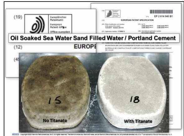
Fig. 10 Titanate modified ordinary Portland cement composition containing oil soaked sea water sand is made compatible in H 2 O.
