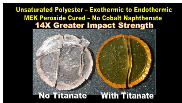
Fig. 18 – Conventional cobalt cure disc fractures while the titanate cured disc broke only after a 2 nd drop from a 6' height.
