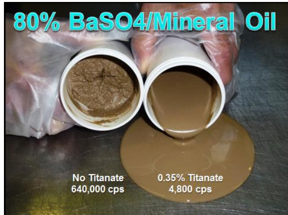
Fig. 7 – Effect of 0.35% titanate on non-Silane reactive 80% BaSO 4 filled non-polar Mineral Oil.
