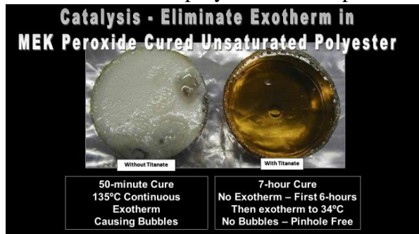
Fig. 17 – The use of a titanate absent cobalt naphthenate slows the cure at 25°C – but eliminates the heat of exotherm and the resultant micro-bubbles. At 40°C, the heat accelerated cure is faster than cobalt.
