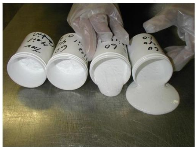
Figure 23— 60% \text{TiO}_2 /min. oil (left to right): no titanate = 512,000 cps; with LICA 38: 0.25% = 128,000 cps; 0.5% = 32,000 cps; 1.0% = 12,800 cps.
