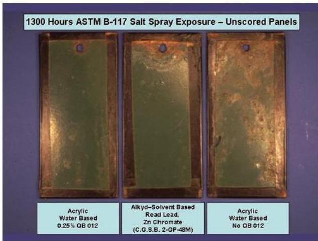
Figure 47—Painted: WB acrylic with QB 012 outperforms acrylic heavy metal alkyd controls.
