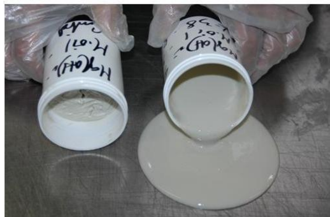
Figure 17—(Left) 50% \text{Mg}(\text{OH})_2 in mineral oil has viscosity of 640,000 cps. (Right) 0.7 wt. % LICA 38 of \text{Mg}(\text{OH})_2 added in-situ to mineral oil followed by \text{Mg}(\text{OH})_2 has 12,800 cps viscosity.
