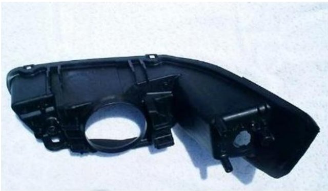
Figure 30—40% FG/Nylon automotive part had a 7-second reduction in cycle time and lowered process temperatures (°C) by 11% (rear zone: 282-248; zone 1: 304-254; zone 2: 304-227; nozzle: 310-260) using 1% CAPS L 44/E titanate added to the IM machine hopper.
