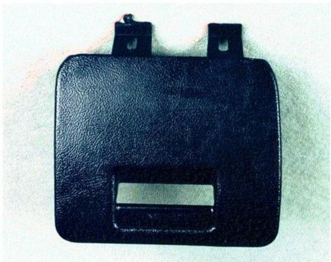
Figure 28—40% FG/PC Ford F-Series Truck Fuse Box Cover-57g shot I.M. with 1% CAPS L 12/L showed: a 60 to 45 sec. cycle reduction; a 52°C temp. reduction; a 45% SPC reduction in out of tolerance measurements; increase in properties: Tensile Strength (54.5 MPa), notched izod (44.6KJ/m 2 ) and MFI (22.9 g/10 min.).
