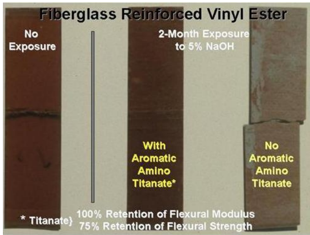
Figure 35—Fiberglass reinforced vinyl ester (Left) No exposure control. (Center) 0.4% of an aromatic amino titanate (LICA 97) shows resistance to 2-month exposure in caustic retaining 100% of Flexural Modulus and 75% of Flexural Strength. (Right) Conventional E-glass without titanate added shows significant aged-deterioration.
