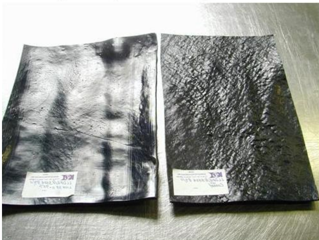
Figure 26—The sheet containing 11% untreated carbon black in 20 MI LLDPE (left) off a two roll mill is rough w. poor appearance while the sheet (right) using the same concentration of 0.75% LICA 38 pretreated carbon black is smoother.
