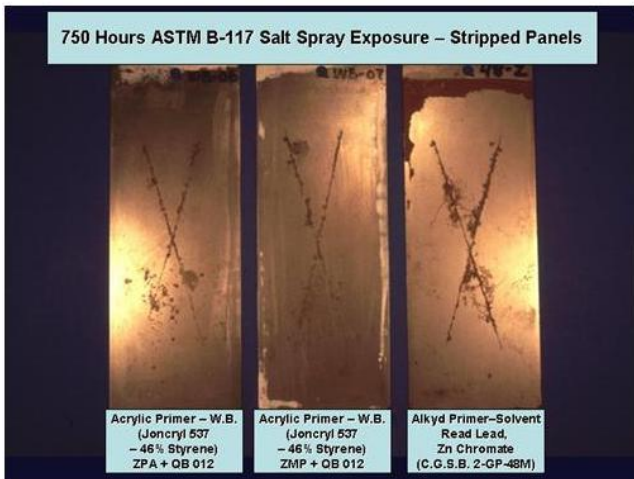
Figure 46—Stripped: WB Acrylic systems with QB 012 titanate quat replace heavy metal alkyd.
