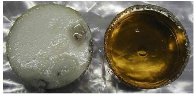
Figure 32—(Left) Control: MEKP cured unsaturated polyester has a 50-minute cure with a 135°C continuous exotherm causing bubbles. (Right) 1% CP-03 hybrid titanate exhibited a 7-hour cure, no exotherm – first 6-hours, then exotherm to 34°C (94°F) exhibiting no bubbles – pinhole free.
