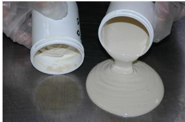
Figure 16—(Left) 40% Calcined Clay in mineral Oil has viscosity of >2,000,000 cps. (Right) 0.7 wt. % LICA 38 of calcined clay added in-situ to mineral oil followed by clay has 9,200 cps viscosity.
