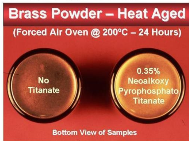
Figure 11—Atomic monolayer of pyrophosphato titanate (KR 38S) provides oxidative protection to heat aged brass metal powder as indicated.
