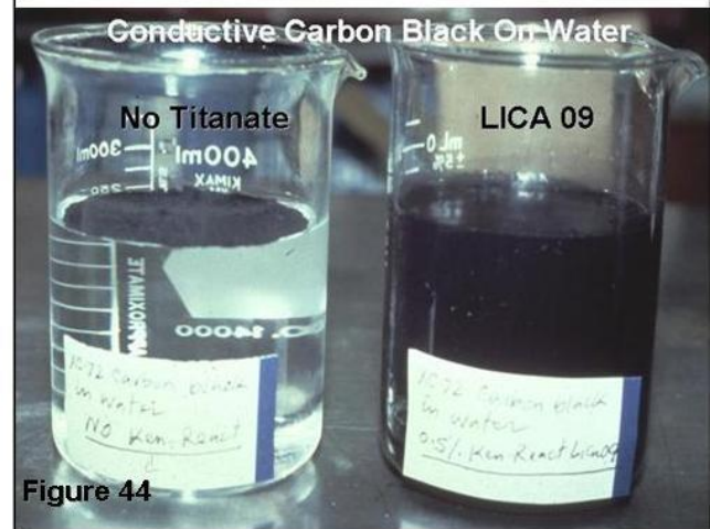
Figures 42, 43 & 44—Carbon Black is rendered water compatible and wettable using water emulsifiable LICA 09. (Top—Middle—Bottom) (Left) Cabot XC-72R carbon black is placed on water and floats. (Right) Time lapse: LICA 09 is emulsified directly into water and begins and instant reaction with the carbon black that causes it to be completely dispersed without any stirring.
