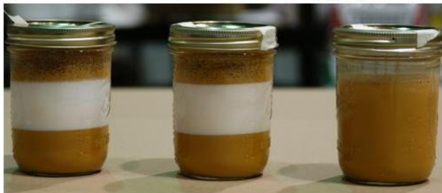
Figure 13—(Left) Ceramic powder into solvated PTFE is not wetted out and phase separates. (Center) The center jar had a neoalkoxy phosphato titanate (NZ 12) dispersed into water/PTFE followed by addition of ceramic. Since the NZ 12 is insoluble in water the ceramic is unwetted and the zirconate gave no benefit. (Right) Organosoluble NZ 12 added to a solvent/PTFE @ RT followed by ceramic creates a stable an homogenous mixture.
