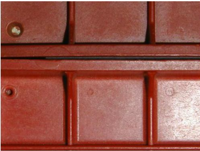
Figure 29—(Top) 40% FG, Fe 2 O 3 filled PC part with poor weld lines (Bottom) 1% CAPS L 12/L titanate allowed: reduction of IM process temps. by 116°C; eliminated weld line problem; improved appearance; and increased impact strength.
