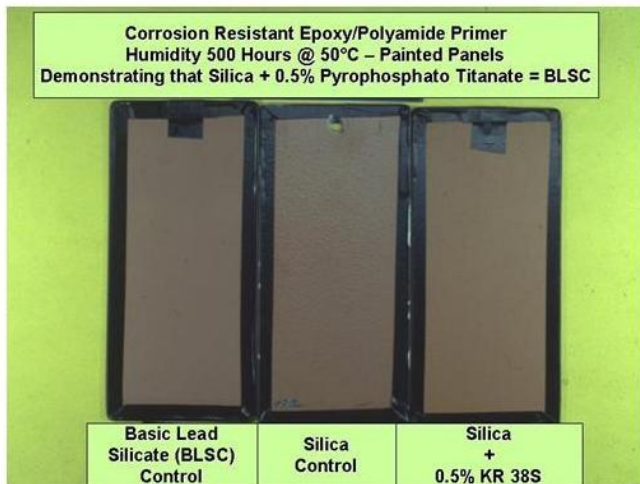
Figure 7—Epoxy/Polyamide Primer—Painted Panels. A test to demonstrate that a pyrophosphato titanate coupled silica can replace BLSC.
