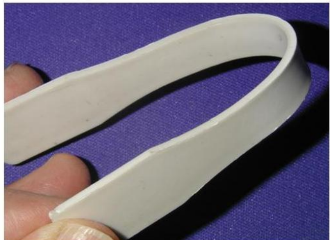
Figure 4—180° bend of 70% 3-micron CaCO 3 , 0.5% KR TTS titanate treated filled PP homopolymer showing rubber-like flexibility and no white stress cracking.
