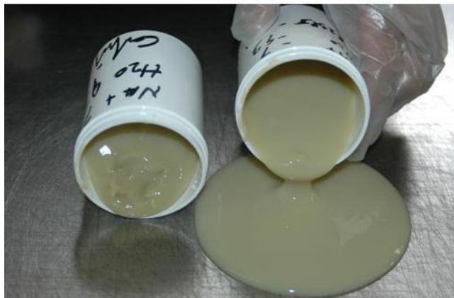
Figure 52—(Left) 7% Cloisite Na+ MMT Nano Clay in Water has 96,000 cps viscosity and shows no flow—had to hit jar several times to make the gel move. (Right) 7% Cloisite Na+ MMT Nano Clay in Water having 5.0 wt. % QB 046 titanate quat added in-situ has 1,400 cps viscosity and flows readily.
