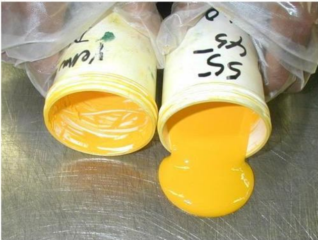
Figure 19—The dispersion effect of 0.5% LICA 38 on 55% PbChromate Yellow/DOP—see Table 10.
