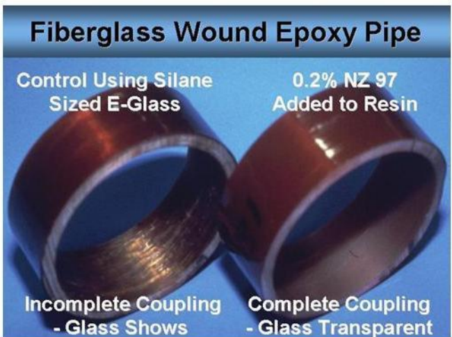
Figure 34—(Left) E-glass fiber wound epoxy pipe with no coupling agents shows glass fibers. (Right) 0.2% of an aromatic amino zirconate (NZ 97) is added directly to the epoxy resin and shows no glass fibers due to coupling in-situ to glass and complete wetting by epoxy.
