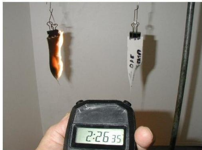
Figure 37—(TOP) Start ignition: (left) 44% \text{CaCO}_3 /LLDPE. (right) 44% \text{CaCO}_3 /3% LICA 38/LLDPE. (BOTTOM) 2 min:26 sec into burn: (left) Burns away completely. (right) 3% LICA 38 titanate/ \text{CaCO}_3 extinguishes the burn.
