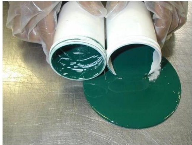
Figure 21—The dispersion effect of 0.5% LICA 38 on 60% \text{Co}(\text{AlCr})_2\text{O}_4 Green (F-5687)/Mineral Oil—see Table 10.
