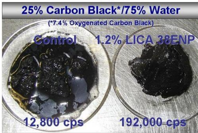
Figure 41—Carbon Black rendered water compatible and wettable with 1.2 wt. % LICA 38ENP .
