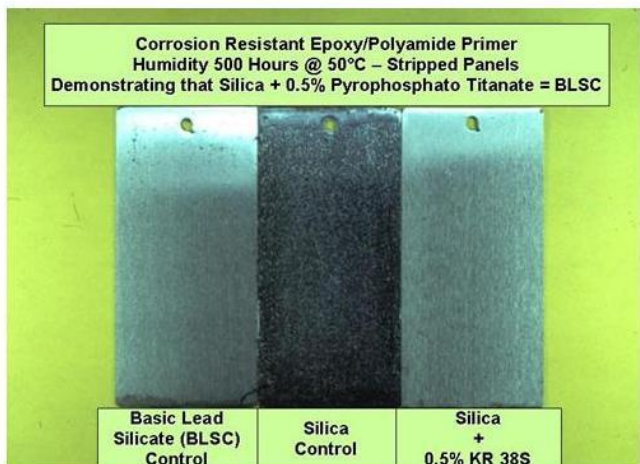
Figure 8—Epoxy/Polyamide Primer—Stripped Panels. Titanate coupled silica can replace BLSC.
