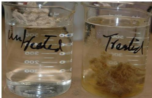
Figure 14—Creafill TC 4005 (Recycled Flax) in water untreated does not wet. (Right) Creafill TC 4005 treated with 2.0% KR TTSWE25 is wetted by water and sinks to the bottom.
