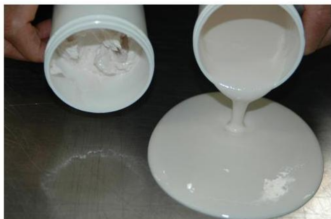
Figure 38—(Left) 60% fine particle ATH in mineral oil has 800,000 cps viscosity and shows no flow. (Right) 60% ATH in mineral oil with 0.7 wt. % LICA 38 added in-situ has 9,600 cps viscosity and flows readily.
