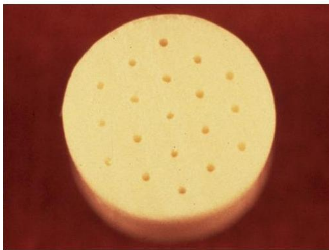
Figure 36—19-Perf. LOVA (LOW Vulnerability Ammunition) 120mm Abrams A1A propellant (85% RDX/CAB) containing 0.5% LICA 12 titanate to: control burn rate & burn rate exponent; couple the RDX to the CAB for better aging; and increase flow of the CAB composite to eliminate “pin drift” during extrusion and maintain concentricity of the perforations.
