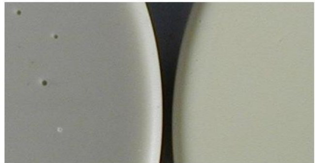
Figure 33—(Left) 3-μ CaCO 3 filled MEKP cured unsaturated polyester casting shows exotherm pinholes. (Right) Hybrid titanate eliminates pinholes.
