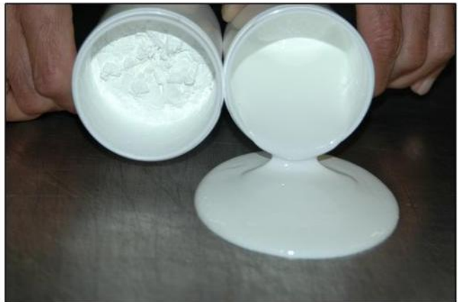
Figure 22—(left) 55% 0.3\mu ZnO in mineral oil has a viscosity of 1,600,000 cps. (Right) 0.5 wt. % LICA 38 of ZnO has 12,800 cps viscosity.
