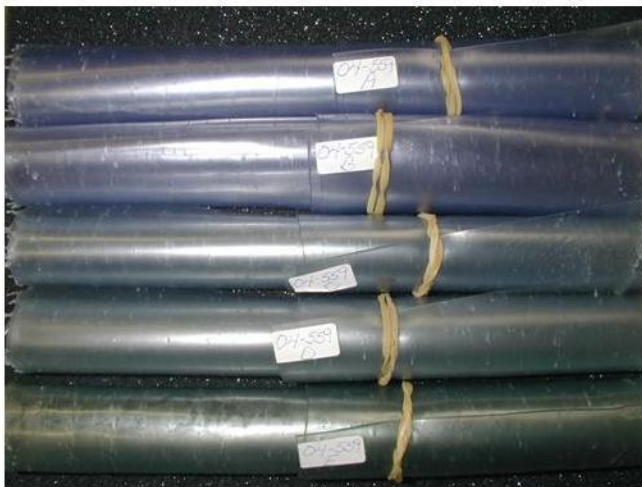
Figure 55—Five transparent sheets of flexible PVC contain a 60% powder masterbatch of a combined dissimilar trineoalkoxy zirconate antistat that forms a nano Zr electron conducting network exhibiting 10^{12} surface resistivity, Ω/sq. and 10^{10} volume resistivity, Ω·cm.—independent of atmospheric moisture.
