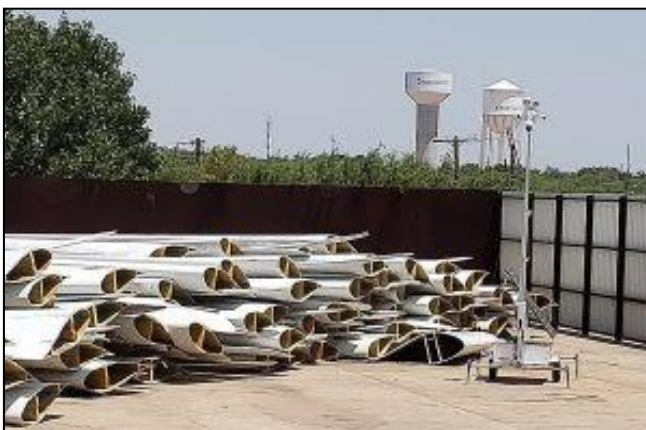
Aged Silane Sized Fiberglass Windmill Blades Headed to Landfill Due to Intefacial Failure
