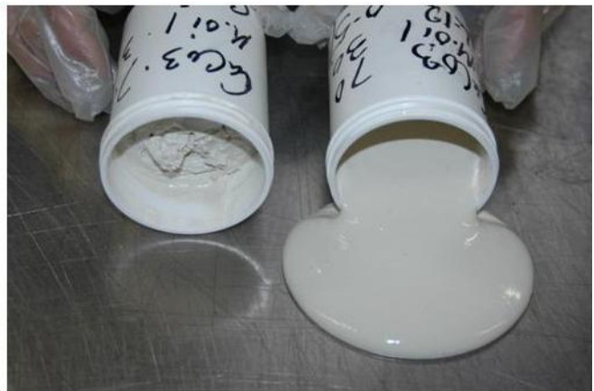
Figure 3—(Left) 70% 3- \mu CaCO 3 in mineral oil has 2,080,000 cps viscosity. (Right) 0.7 wt. % LICA 38 of CaCO 3 added in-situ to mineral oil followed by 70% 3-mircon CaCO 3 has 12,800 cps viscosity.
