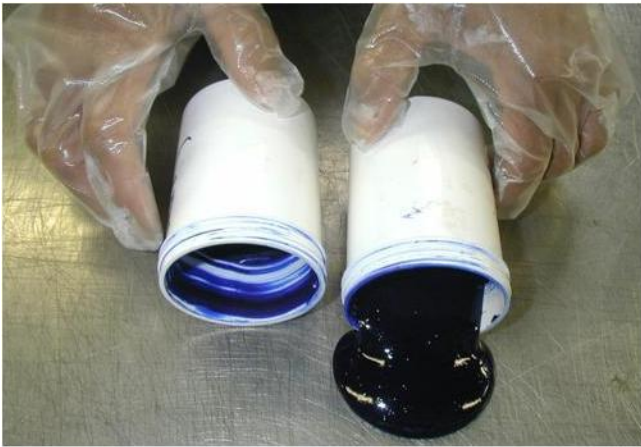
Figure 18—The dispersion effect of 0.5% LICA 38 on 55% ultramarine blue (Holliday 51-51)/DOP—see Table 10..
