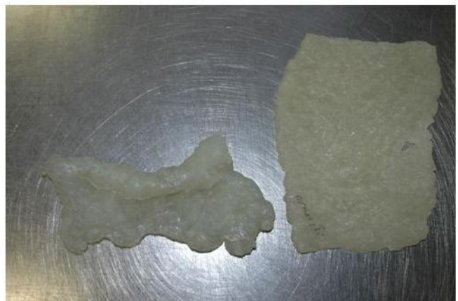
Figure 5—Nervy unfilled EPR (left). EPR derived with 0.2 phr phosphato titanate (right) indicating Function 2 polymer flexibilization.
