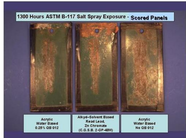
Figure 48—Scored: WB acrylic with QB 012 outperforms acrylic heavy metal alkyd controls.
