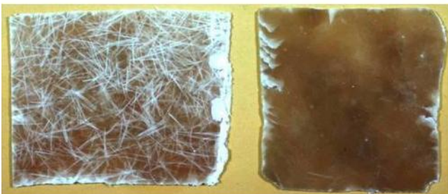
Figure 31—(Left) FG (silane sized E-glass)/MEKP cured unsaturated polyester shows glass fibers. (Right) titanate composition does not show fibers.
