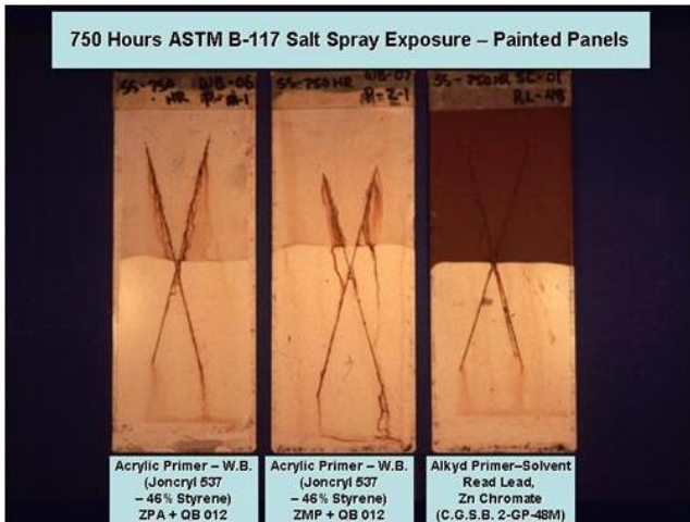
Figure 45—Painted: WB Acrylic systems with QB 012 titanate quat replace heavy metal alkyd.
