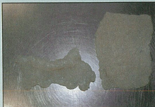
Figure 10 - 44% CoCO_3 /LLDPE compound without pyrophosphato titante burns to clip after 2 min. 37.53 sec. (left) - 3% pyrophosphato titanate extinguishes burn
