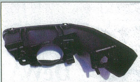
Figure 14 - the 40% FG/nylon automotive part shown had a seven-second reduction in cycle time and lowered process temperatures (°C) by 11% (rear zone: 282-249; zone 1: 304-254; zone 2: 304-227; nozzle: 310-260) using 1% of a 20% active amino titanate pellet masterbatch dispersed in EVA
