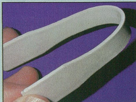
Figure 4 - 0.5 wt. % KR TTS titanate flexibilizes 70% 3-micron \text{CaCO}_3 filled polypropylene homopolymer
