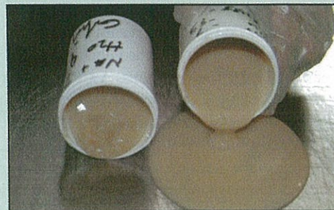
Figure 8 - 7% Cloisite Na + MMT nano clayin water - 96,000 cps (left) - 5% pyrophosphato titanate quat - 1,400 cps (right)
