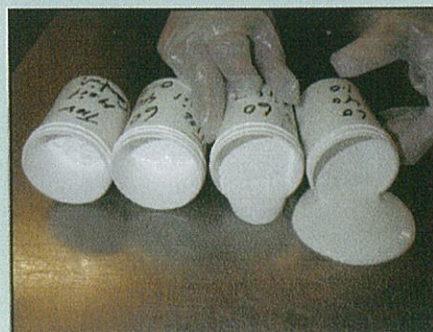
Figure 12 - 60% TiO 2 /mineral oil - no titanate (left); 0.25% (left-center); 0.5% (right-center); 1.0% (right)
