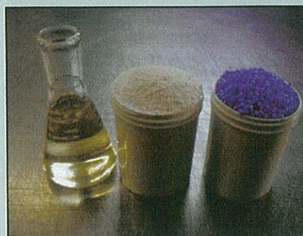
Figure 11 - titanate forms: 100% active liquid; 65% active powder; 20% active pellet
