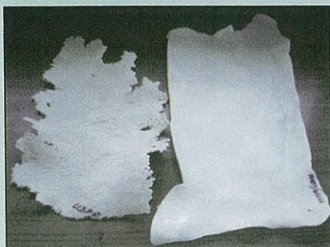
Figure 6 - 60% Mg(OH) 2 filled 20 M.I. LLDPE - no titanate (left) and 0.7% pyrophosphato titanate (right)
